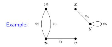
Here, the vertices are  $V=\{u,v,w,x,y\}$ , and the edges are  $E=\{e_1=u-v,\ e_2=u-w,\ e_3=u-w,\ e_4=x-y,\ e_5=y-y\}.$  An edge that connects a vertex to itself (like  $e_5$ ) is called a loop. We say a vertex a is adjacent to a vertex b if there is an edge connecting a and b. (Notice that for a generic graph, "adjacency" is a symmetric relation, but is not reflexive nor is it transitive.)
