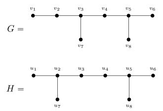
Both of these graphs have the degree sequence 3,3,2,2,1,1,1,1. But in G, there's a vertex of degree 1 adjacent to a vertex of degree 2, where as no vertex of degree 1 is adjacent to a vertex of degree 2 in H. So  $G \ncong H$ .
