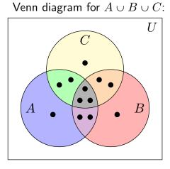
$$\begin{split} |A \cup B \cup C| &= |A| + |B| + |C| & \text{``include''} \\ &- (|A \cap B| + |A \cap C| + |B \cap C|) & \text{``exclude''} \\ &+ |A \cap B \cap C|. & \text{``include''} \end{split}$$
