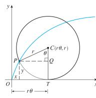
Parameter:  $\theta$ , the rot'l angle of circle. Center: The edge of the circle has all touched the ground. So the distance of the center from the y-axis is the arc length of the circle with angle  $\theta$ . So the center is at  $C=(r\theta,r)$ .
