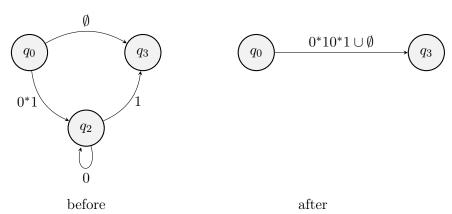
So the transition from  $q_0$  to  $q_3$  is labeled with  $0*10*1 \cup \emptyset$ , which simplifies to 0\*10\*1. (d)
