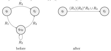
Letting  $q_i = q_0$ ,  $q_j = q_3$ , and  $q_{\text{rip}} = q_2$ , identify  $R_1, R_2, R_3$  and  $R_4$ . What regular expression labels the transition from  $q_0$  to  $q_3$  after ripping out  $q_2$ ? What obvious simplification can you make involving the empty set?
