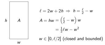
Since the interval  $[0, \ell/2]$  is closed and bounded and A is continuous, the extreme value theorem says that A has a maximum on this interval.
