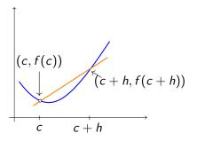
The slope of the orange secant line is  $\frac{f(c+h)-f(c)}{h}$ .
