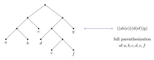
**Full binary tree to balanced parenthesization.** To form the corresponding balanced parenthesization, we label each left edge with a "(" on its left and a ")" on its right. We then take a clockwise trip around the tree, hugging close to the edges and reading off the labels (the dashed line gives a hint of the path):
