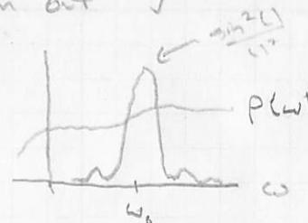
$$P(t) = \frac{2|\mathbf{p}|^2}{\hbar^2} \int_0^\infty \frac{\sin^2((\omega_0 - \omega)t/2)}{(\omega_0 - \omega)^2} d\omega$$
