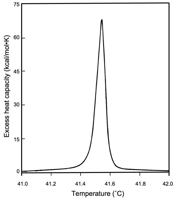
Differential scanning calorimetry scan of dipalmitoylphosphocholine in water. The transition temperature is 41.5°C. (Figure adapted from Albon & Sturtevant (1978) *Proc. Natl. Acad. Sci. USA* **75**, 2258-2260).
