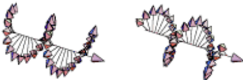
Figure CD.3 Two photons of opposing spin. Each line perpendicular vector to the line of travel represents the position of the electric field vector at one given time. Note that the side on view would appear to be an oscillating wave.
