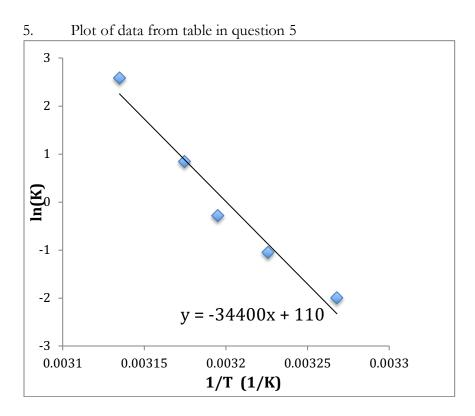
Note that  $\Delta H = -\text{slope} * R = (-34400 \text{ K}^{-1})(0.001987 \text{ kcal/molK}) = 67 \text{ kcal/mol}$  $\Delta S = \text{intercept} * R = 110(1.987 \text{ cal/molK}) = 220 \text{ cal/molK}$
