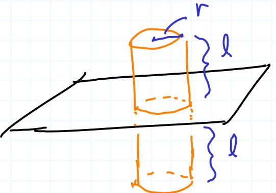
Consider a cylinder through the plane, as shown. We've chosen a circular cylinder, but that's not important. By symmetry, we'll assume  $E$  has no flux through the sides of the cylinder and that  $E$  is perpendicular to the top and bottom of the
