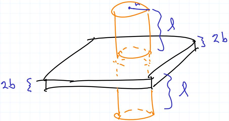
$$\text{flux through cylindrical surface at distance } l \text{ from plate} = |E(l)| (\pi r^2 + \underbrace{\pi r^2}_{\text{top}} + \underbrace{\pi r^2}_{\text{bottom}}) = 2|E(l)|\pi r^2$$
