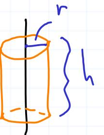
$$\begin{aligned} \text{Flux} &= |E(r)| 2\pi r h \\ &= \text{enclosed charge} (\epsilon_0 = \lambda h / \epsilon_0) \end{aligned}$$
